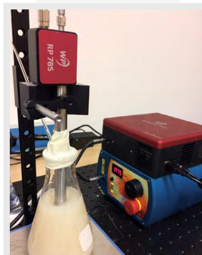
Figure 2: Fermentation Setup (front) on magnetic stirrer (bottom) with probe (top) and spectrometer and laser (back).
