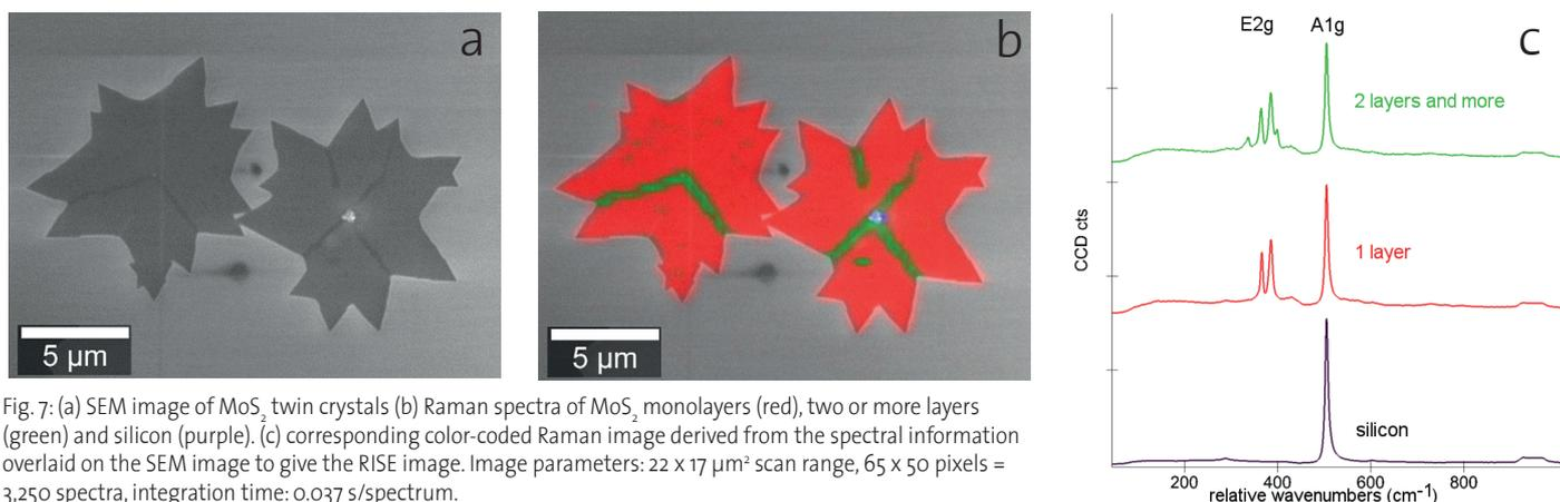
Fig. 7: (a) SEM image of MoS<sub>2</sub> twin crystals (b) Raman spectra of MoS<sub>2</sub> monolayers (red), two or more layers (green) and silicon (purple). (c) corresponding color-coded Raman image derived from the spectral information overlaid on the SEM image to give the RISE image. Image parameters: 22 x 17 μm<sup>2</sup> scan range, 65 x 50 pixels = 3,250 spectra, integration time: 0.037 s/spectrum.
