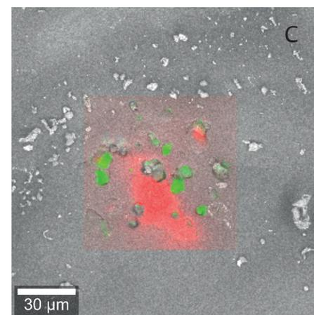
Fig. 5: (a) Characteristic Raman spectra of SWCNTs and PE. (b) color-coded Raman image. (c) RISE image. Image Parameters: 150 x 150 μm<sup>2</sup> scan range, 80 x 80 pixels = 6,400 spectra, integration time: 60 ms/spectrum, PE (red), SWCNTs (green), SEM image (grey).
