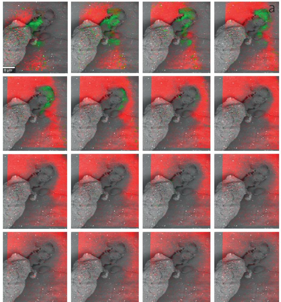
Fig 6: 3D imaging of SWCNTs on PE film. For a 3D image of the SWCNTs on PE sample 16 equidistant Raman images were taken while the focus was shifted by 1  $\mu\text{m}$  for each image. The individual images are displayed as RISE images in (a). The compiled 3D Raman image of the analyzed sample area shows the SWCNTs located on the top of the PE filter (b).
