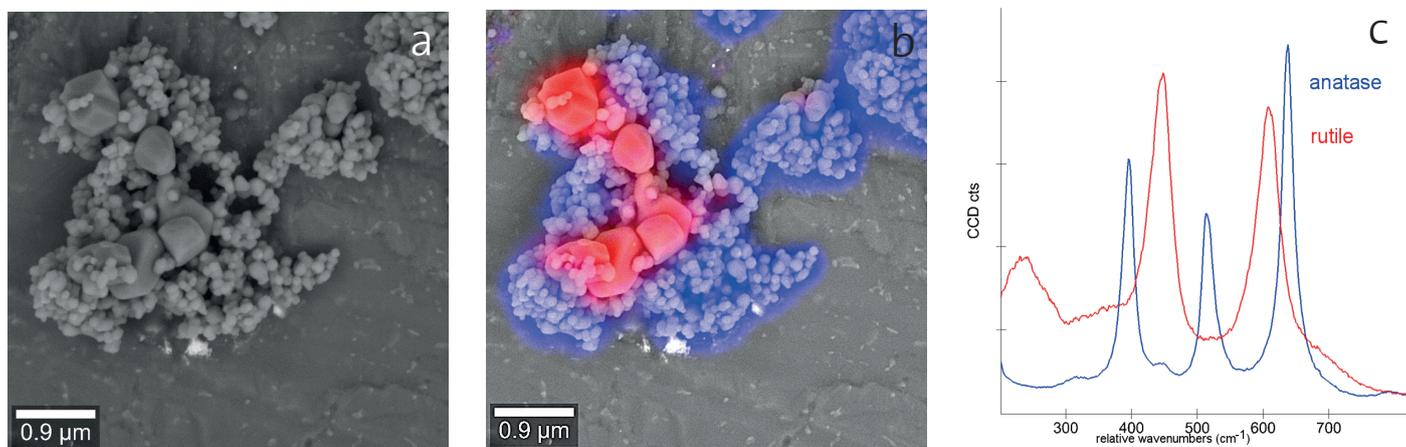
Figure 8: Two modifications of TiO<sub>2</sub>, anatase and rutile, were mixed 1:1, ground, dissolved in water and imaged with an SEM (a) and a confocal Raman microscope. (b) SEM and Raman images overlaid. (c) In the Raman spectrum anatase (blue) can be easily distinguished from rutile (red). Image parameters: 12 x 12 μm<sup>2</sup> scan range, 150 x 150 pixels = 22,500 spectra, integration time: 0.037 s/spectrum.
