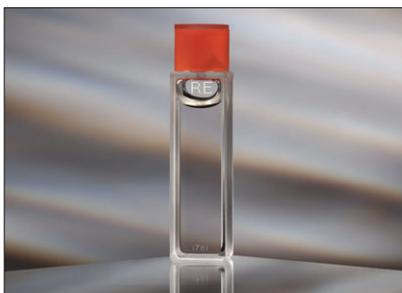
**Figure 1.** Sealed certified wavelength reference.
