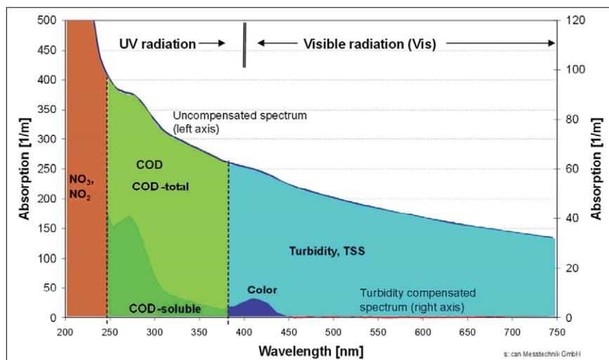
**Figure 2.** UV/vis spectrum and examples of parameters derived out of this spectrum together with their characteristic absorbance profiles. [chemical oxygen demand (COD); total suspended solids (TSS)].
