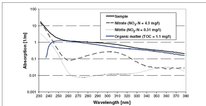
**Figure 3.** UV spectrum for tap water spiked with nitrite and deconvolution into spectra of nitrate, nitrite and organic matter.<sup>2</sup>
