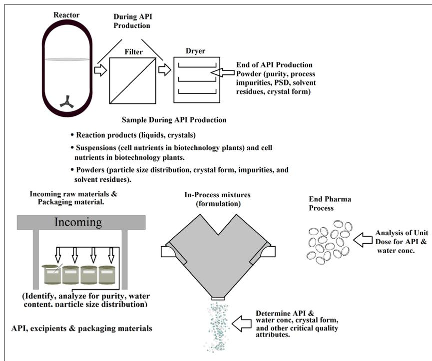
**Figure 2.** Flow path of the generic pharmaceutical manufacturing process with the principal sampling locations indicated taken from Reference 5 with permission.
