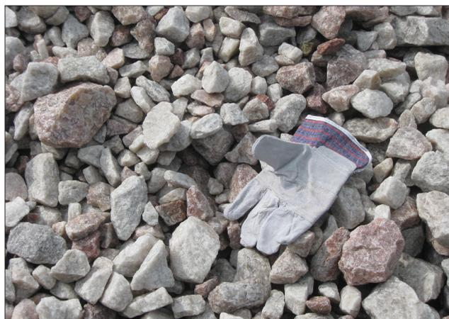
Close-up of the typical dimensional manifestation of quartzite blocks (safety glove for scale). Block surface flatness, which influences the quality of HHXRF analysis, is commented upon further in the text.
