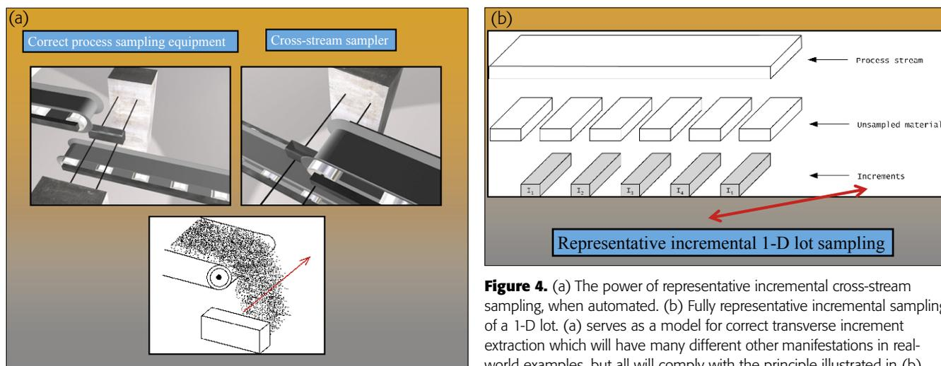
**Figure 4.** (a) The power of representative incremental cross-stream sampling, when automated. (b) Fully representative incremental sampling of a 1-D lot. (a) serves as a model for correct transverse increment extraction which will have many different other manifestations in real-world examples, but all will comply with the principle illustrated in (b).
