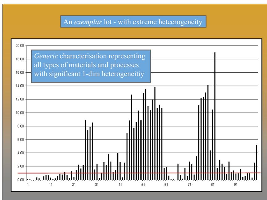
**Figure 5.** Representative extraction [cf. Figure 4(b)] of 100 increments of a 1-D process stream reveal a pressing need for an effective composite sampling scheme if one is to be able to state with any reliability an average concentration of the 100 individual analytical results presented. It turns out (see later columns) that the pertinent  $Q$  for this difficult task is  $Q=42$ . [For the reader who cannot wait, this example derives from the famous KeLDA study (see Literature).]
