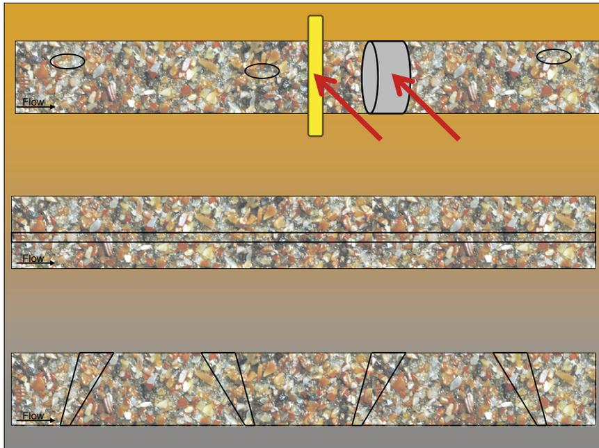
**Figure 2.** Increments can be extracted from 1-D lots in a variety of ways, but only one is correct (representative): a complete slice of the stream/flow defined by parallel boundaries (shown in yellow). All other increment delineations shown are incorrect and will give rise to a sampling bias. For process sampling, e.g. a pipeline, the correct increment delineation is also a planar-parallel slice of the flow, i.e. a cylindrical cut (shown in grey).
