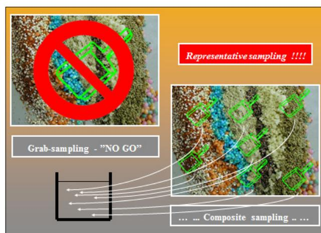
**Figure 4.** Composite sampling ( $Q = 7$ ) does a much better job than a single grab sample of the same mass/size. FSP-compliant composite sampling is the only way towards representative sampling, and is in fact only dependent upon the magnitude of  $Q$ —the more (smaller) increments the better.
