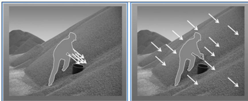
**Figure 3.** Local vs broad deployment of the same number of increments,  $Q$ . Note, however, that while the broadened-out deployment plan in the right panel does a much better job of “covering” the surface of the lot, it does not sample from within the significantly larger inner volume? How to “cover” a full-fledged 3-D lot?
