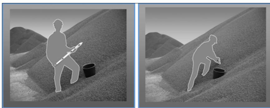
**Figure 1.** A single grab sample (specimen) is never able to represent the entire lot because it is manifestly not able to cover any material with a significant heterogeneity (compositional heterogeneity and distributional heterogeneity). This important truth holds for lots of *all* sizes, shapes and forms.
