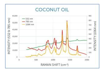
Figure 3: Raman spectrum of coconut oil compared using different excitation wavelengths: 532 nm (green line), 785 nm (red line) and 1064 nm (yellow line)
