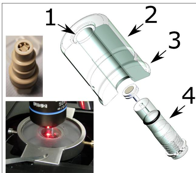
**Figure 1.** Compact confinement for Raman investigation of nuclear material. 1: optical window, 2: acrylic glass cylinder capsule. 3: flange for the fixation of the plastic bag tunnel. 4: movable sample support. Down left the confinement installed under a microscope. Up left: movable sample support for fluid-cell Raman spectroscopy.
