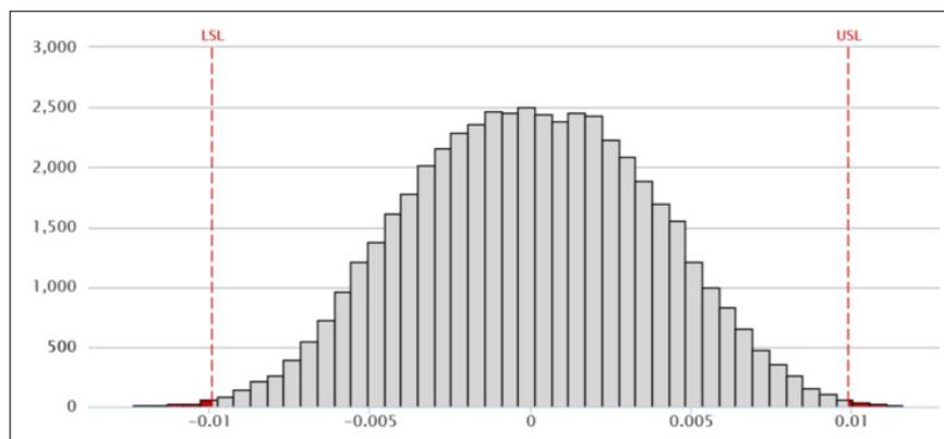
**Figure 2.** Minitab Devize MCS model output for absorbance accuracy acceptance limits of  $\pm 0.0099$  for  $N = 50,000$ .
