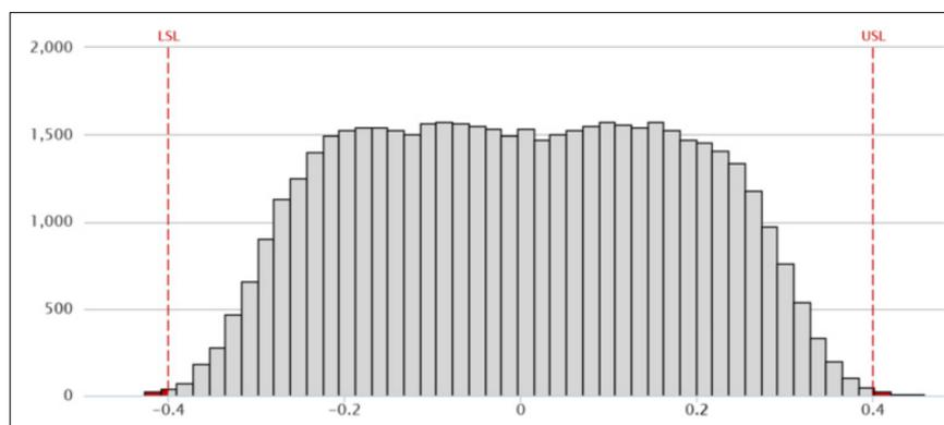
**Figure 3.** Minitab Devize MCS model output for wavelength accuracy acceptance limits of  $\pm 0.4$  nm for  $N = 50,000$ .
