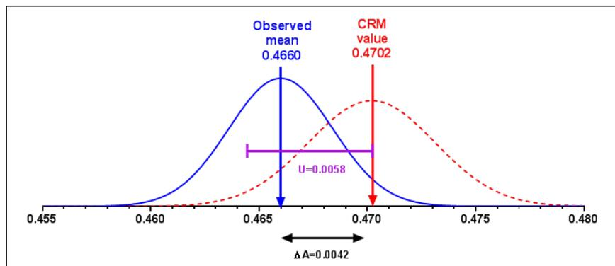
**Figure 1.** An example of a mean measured absorbance value lying inside the combined measurement uncertainty of the measurement and the CRM.<sup>1</sup>
