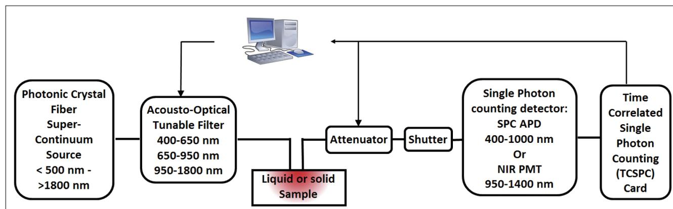
**Figure 1.** The schematic of a typical PToF spectrometer setup.
