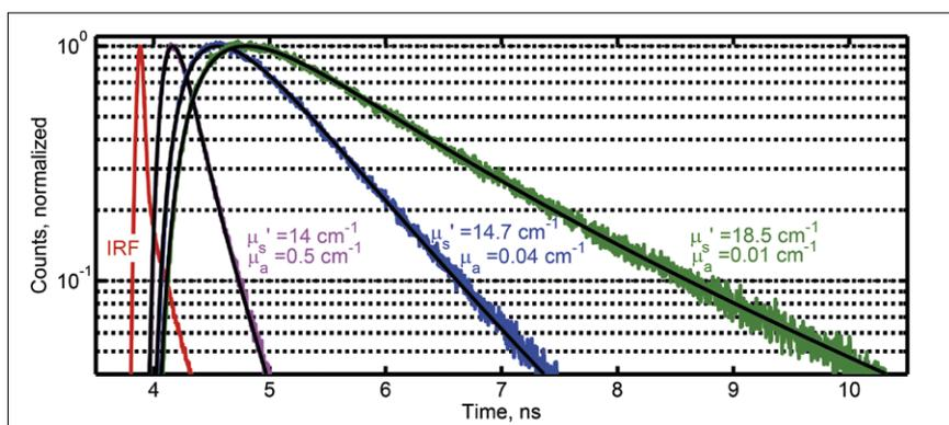
**Figure 2.** PTOF distributions at 700 nm, 830 nm and 980 nm in a 1.5% fat content milk sample plotted as green, blue and magenta lines, respectively. The probe pulse at 980 nm, (IRF, red). Experimental data fits are plotted as black lines.
