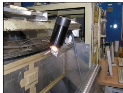
**Figure 2.** Installation of the probe head on a pilot-scale roll coating machine at IOM.
