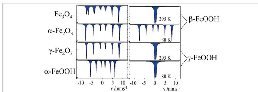
**Figure 10.**  $^{57}\text{Fe}$  Mössbauer spectra of various corrosion products of iron which may be formed under different conditions (reproduced from Reference 17 with permission).
