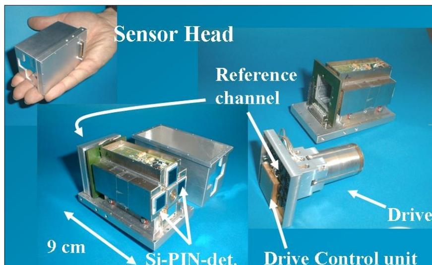
**Figure 12.** The sensorhead of the miniaturised Mössbauer spectrometer, MIMOS II, contains the drive unit, the Mössbauer source and the detectors and amplification electronics (adapted with permission from Reference 8).
