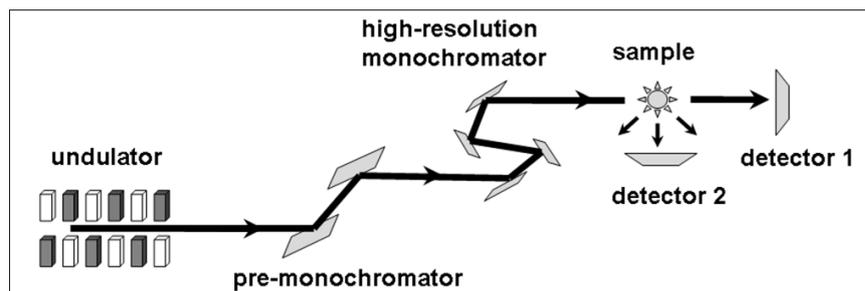
**Figure 15.** Set-up for Nuclear Forward Scattering (NFS) and Nuclear Inelastic Scattering (NIS). For NFS coherent scattering is detected by detector #2 and for NIS incoherent scattering is detected by detector #1 (adapted with permission from Reference 8).
