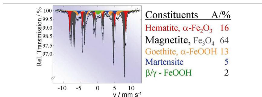
**Figure 11.** Routine Mössbauer analysis of finely dispersed corrosion particles formed in the cooling system of a power plant (reproduced from Reference 17 with permission).
