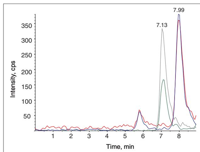
**Figure 3.** API 2000 system: standard with 100 pg absolute: 2-NBA-SEM 209/166 (blue), 209/192 (red), 2-NBA-AHD 249/178 (green), 249/134 (grey).
