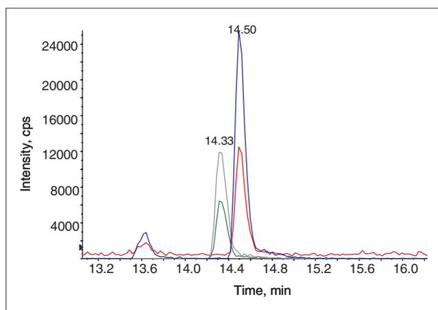
**Figure 2.** API 4000 system; standard with 100 pg absolute: 2-NBA-SEM 209/166 (blue), 209/192 (red), 2-NBA-AHD 249/178 (green), 249/134 (grey).
