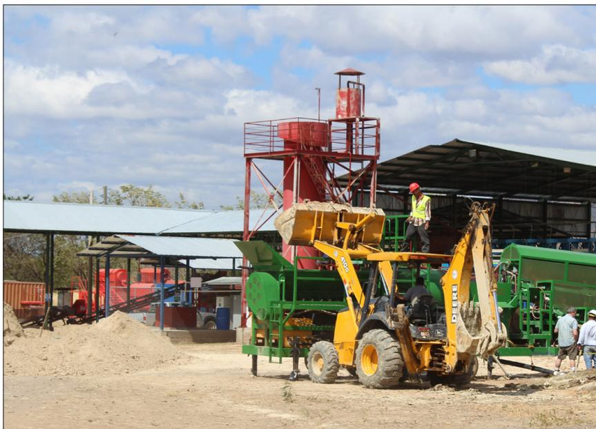
**Figure 5.** Mercury Recovery Plant (MRP) being loaded with tailings (Nicaragua). Reproduced from Reference 7 with permission.
