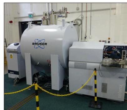
**Figure 1.** FT-ICR mass spectrometer used by the authors.
