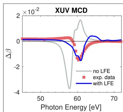
Measured and calculated dichroic absorptive part  $\Delta\beta$  of the magneto-optical function of Cobalt. Including local field effects (LFE) and many-body corrections brings the fully *ab initio* theory into very good agreement with experiment.
