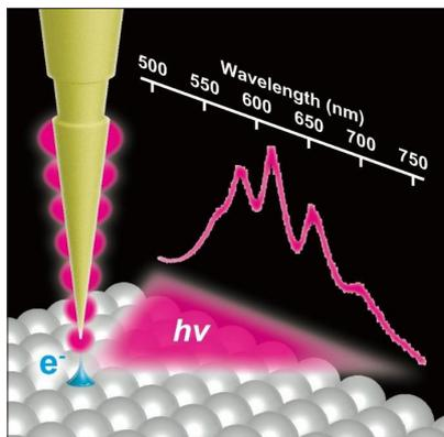
Nanolight (localised surface plasmon) is excited in the STM junction by tunnelling electrons ( $e^-$ ). The emitted light ( $h\nu$ ) shows a modulated spectrum resulting from a Fabry–Pérot interference of the propagating surface plasmon polariton on the shaft. Credit: Takashi Kumagai
