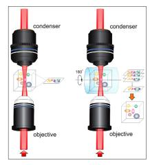
This schematic depicts an imaging system that uses a special type of laser beam called a Bessel beam that is produced using a pair of cone-shaped "axicon" lenses combined with a microscope objective. Purdue University researchers are using the system, which is able to penetrate deep into tissue and might lead to technologies that eliminate the need to draw blood for analyses including drug testing and early detection of diseases such as cancer and diabetes. (Purdue University photo/Ji-Xin Cheng)
