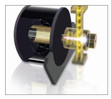
The FLUTE linear accelerator accelerates electron clouds in order to generate terahertz rays. (Illustration: KIT)
