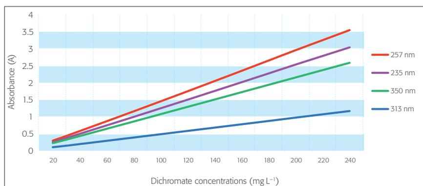
Figure 3. Potassium dichromate linearity.
