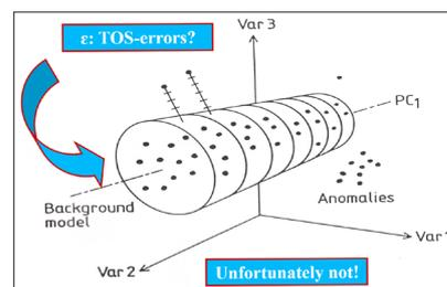
**Figure 7.** Chemometric bi-linear data model of pervasive data structures, PCA or PLS-components (schematic sketch). The multivariate data model errors ( $\epsilon$ s) are often optimistically thought of as “TOS-errors” ( $TSE_{TOT} + TAE$ ), but they are not, see text for clarification.
