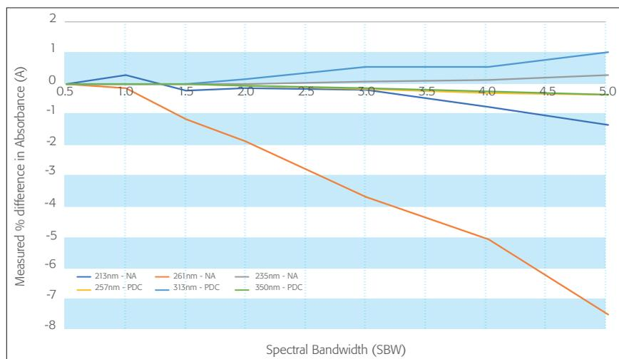
**Figure 1.** Effect of spectral bandwidth on measured absorbance values of nicotinic acid and potassium dichromate solutions. Nicotinic acid (NA) @ 213 nm and 261 nm vs acidic potassium dichromate (PDC) solution @ 235 nm, 257 nm, 313 nm and 350 nm.
