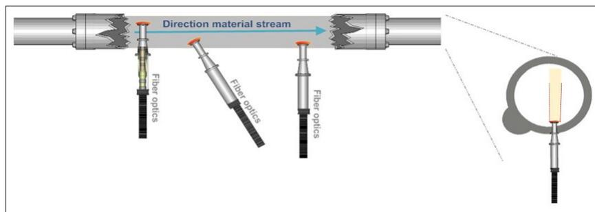
**Figure 2.** The “PAT sensor application solves all sampling issues” fallacy, which follows because PAT sensors are not “seeing” a volume corresponding to a full cross-sectional slice of a moving stream of matter, see also Figure 3. Illustration copyright KHE Consulting and Martin Lischka, reproduced with permission.
