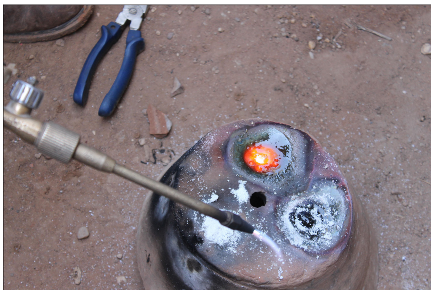
Figure 2. Gold has been concentrated and smelted to a small bead. Reproduced from Reference 7 with permission.
