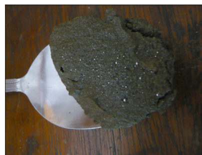
Figure 3. Mercury flour (droplets) in a spoonful of tailings (Philippines). Reproduced from Reference 7 with permission.
