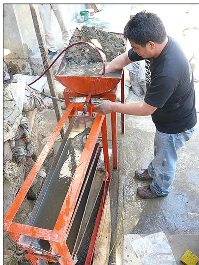
Figure 4. Prototype of “Peter Plates” in action (Philippines). Tailing slurry from the tub is passed over the plates in succession. Reproduced from Reference 7 with permission.
