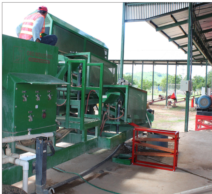
Figure 6. Mercury Recovery Plant (MRP) hooked up with Peter Plates (Nicaragua). Reproduced from Reference 7 with permission.
