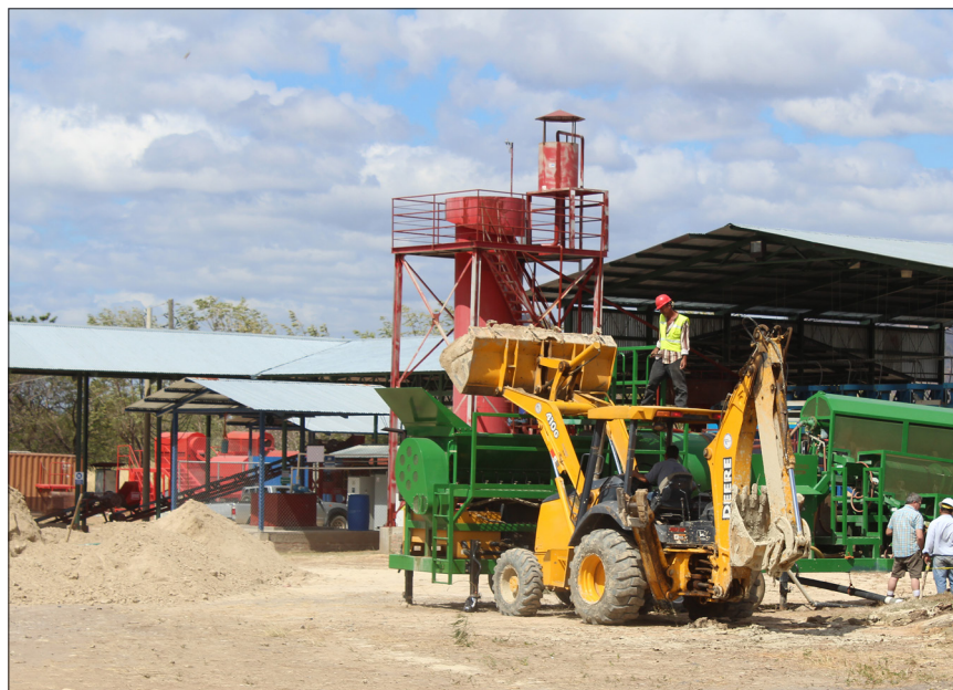
Figure 5. Mercury Recovery Plant (MRP) being loaded with tailings (Nicaragua). Reproduced from Reference 7 with permission.
