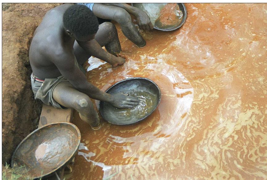
Figure 1. Hand-mixing mercury with milled gold ore (Tanzania). Reproduced from Reference 7 with permission.
