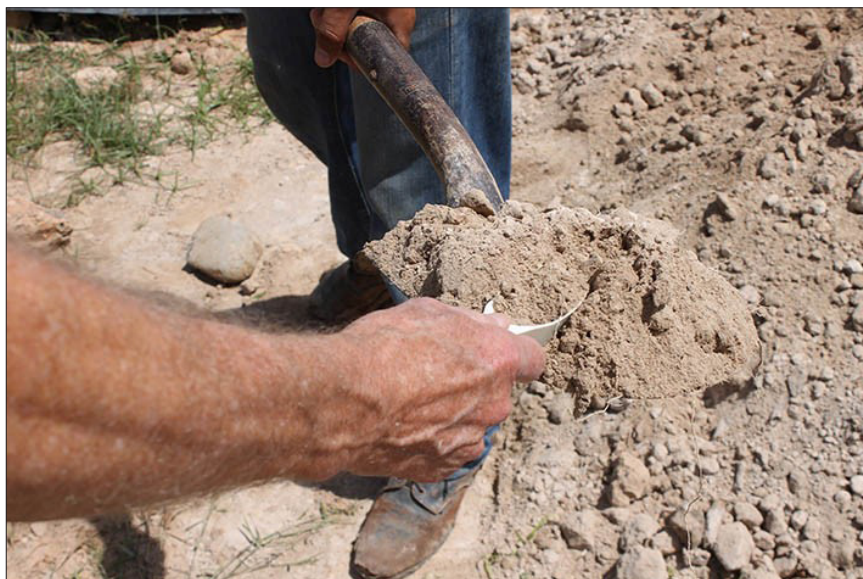
Figure 8. Incremental composite sampling from each shovel used to transport the original lot, see Figure 7. Reproduced from Reference 6 with permission.
