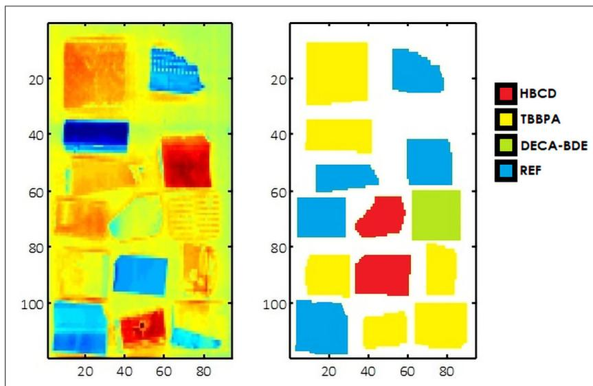
Near infrared hyperspectral imaging of samples of plastics and their classification as a function of type of flame-retardant: 1,2,5,6,9,10-hexabromo-cyclododecane, HBCD (red samples); 3,5-tetrabromobisphenol A, TBBPA (yellow samples); Pentabromophenyl ether, Deca-BDE (green samples); and reference, REF (blue samples).
