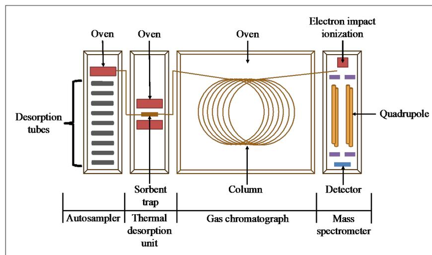
**Figure 1.** Illustration of various steps of thermal desorption hyphenated to gas chromatography/mass spectrometry, adapted and modified from Materic *et al.*<sup>7</sup>
