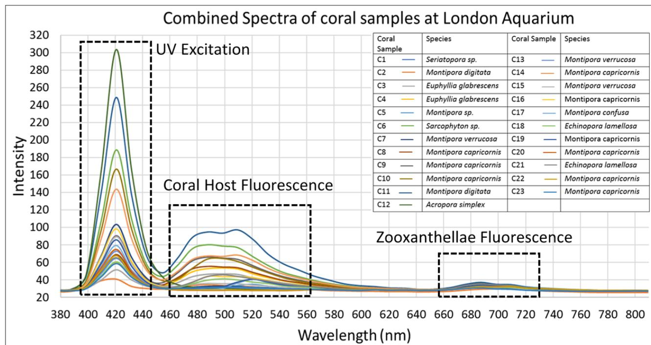
**Figure 2.** A combined plot of spectra generated from hyperdata generated from areas of interest highlighting all fluorescence visible. Areas of UV excitation and coral and zooxanthellae fluorescence are highlighted.
