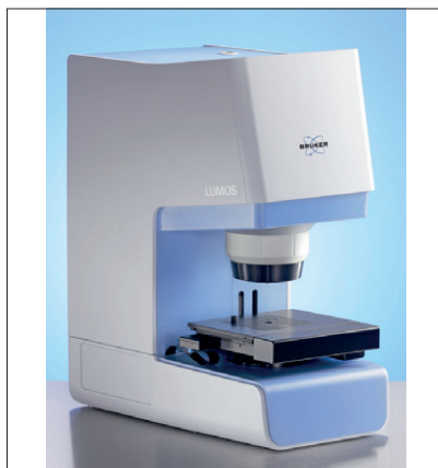
Figure S1. Example of a fully automated FT-IR microscope (Bruker, LUMOS system), which includes a motorized ATR crystal within the objective.
